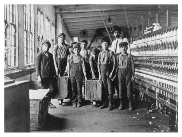
Note: When a bobbin is filled, the "doffer boy" comes along, takes it off the spinning frame and puts an empty bobbin in its place.
